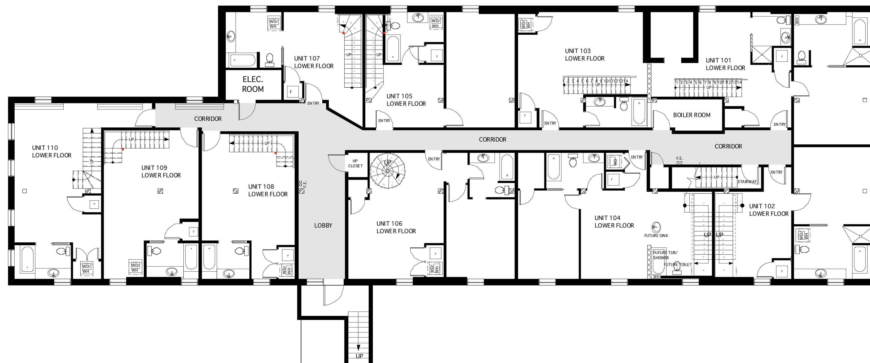
LOWER FLOOR TENANT IMPROVEMENT PLAN Scale: 1/8" = 1'-0"
